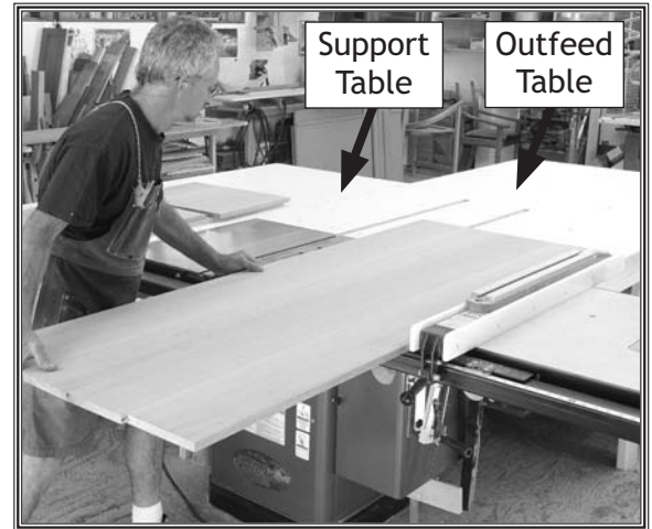
Figure 88. Example of outfeed & support tables.
